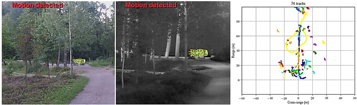
Figure 7: People detection from optical (left) and thermal data (middle). Radar-based detection trajectories (right) with image courtesy of INRAS and Johannes Kepler Universität Linz.
