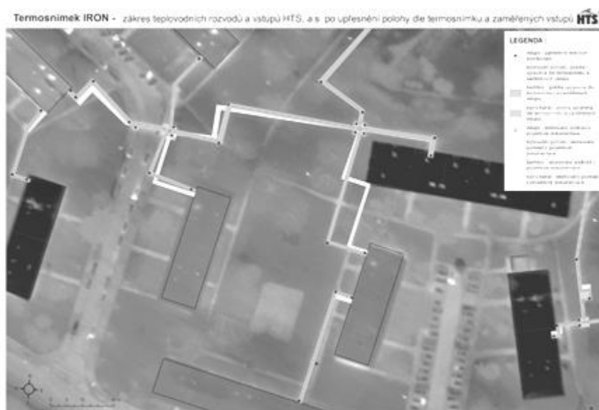
Figure 5 Correction of the documentation in the GIS system using thermal imaging [Author: Moravec]
