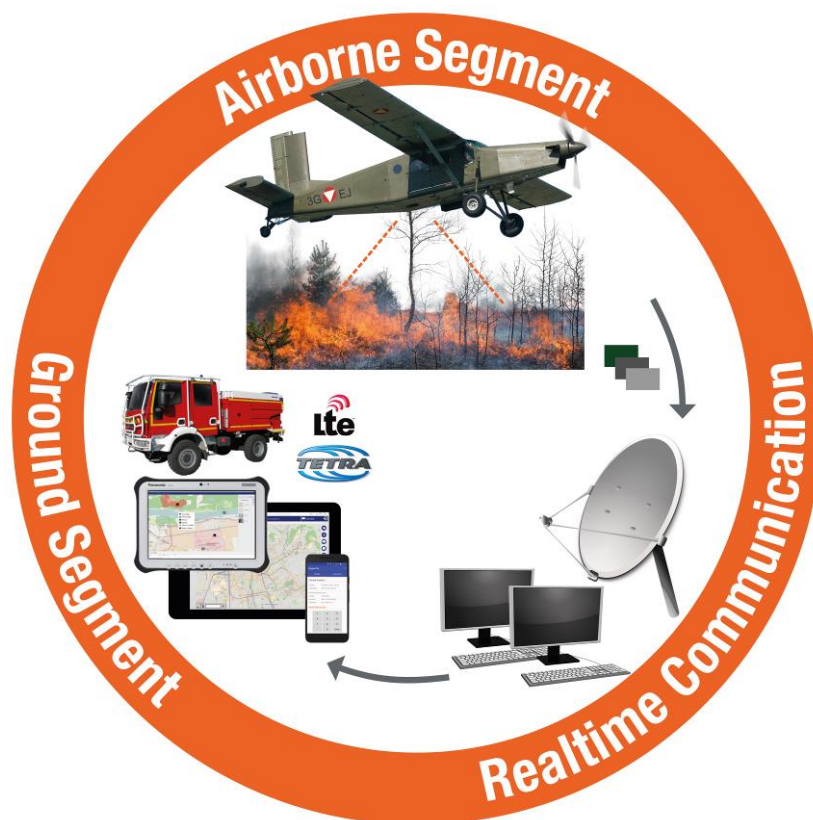
Figure 3: System overview and general concept of data/information flow in a forest fire event situation.
