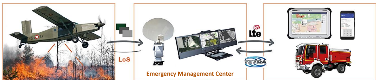
Figure 5: General concept of data acquisition, line of sight (LoS) real-time data communication, data processing and information distribution to support time critical decision processes in forest fire situations (graphic: JOANNEUM RESEARCH)
